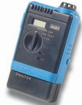
Therefore the Dositox is programmed to start an averaging interval whenever the TLV value is exceeded. This allows the best possible exposure determination for increased safety.
